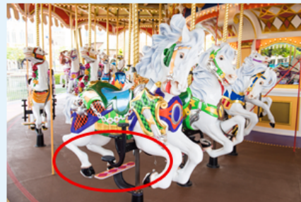
The length and width of the stirrups were extended and more visible paint colors were adopted.
