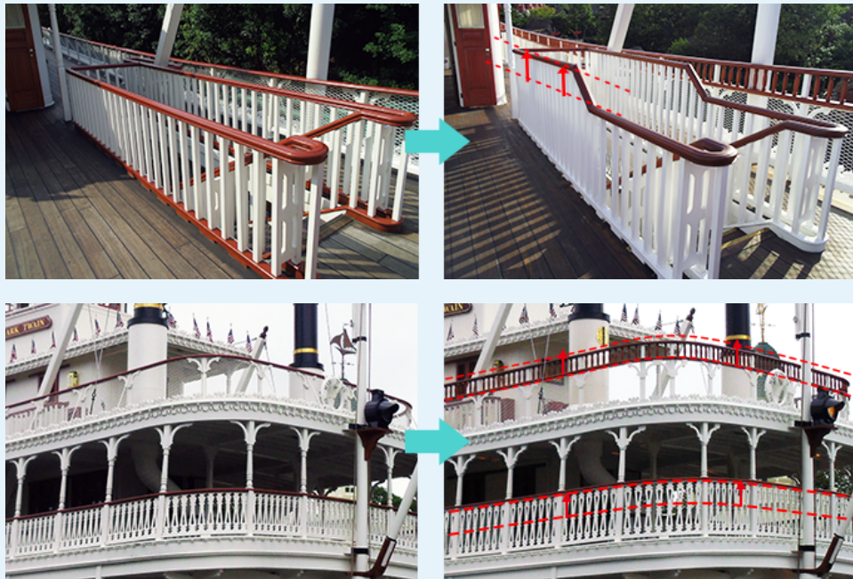
Increased the height of the rails on Mark Twain Riverboat
